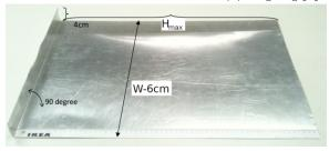
(c) Bending the aluminimum plate
