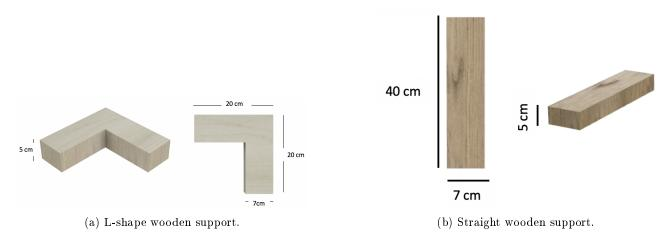
Figure 12: Different support options for the Parkour platform.
