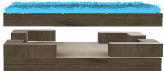
(b) Lower and upper platform with Option 1 L-shape wooden supports for increasing height.
