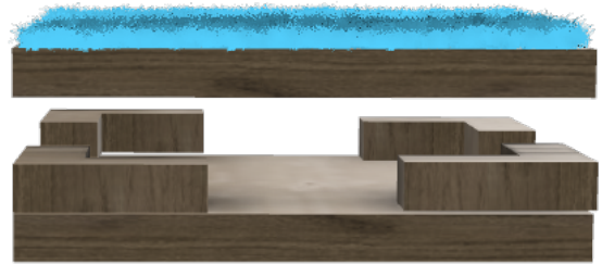
(b) Lower and upper platform with Option 1 L-shape wooden supports for increasing height.
