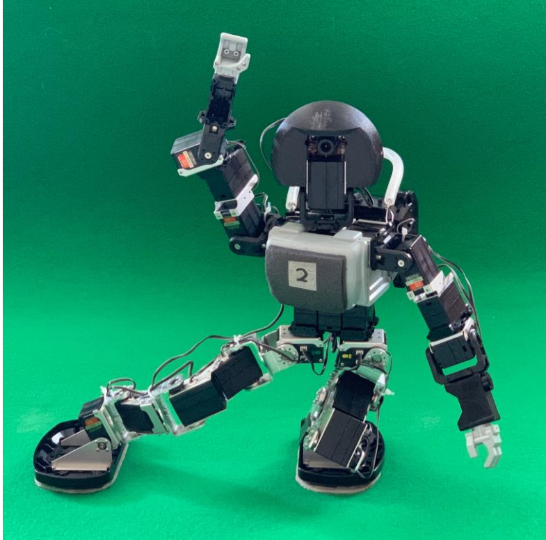
Kondo robot upgraded with smart camera
