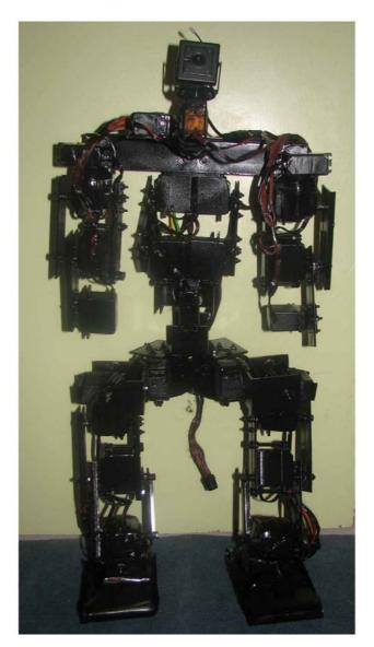
Number of degrees of freedom : 120 degrees Type of motors : Servomotor Computing Unit : Laptop Camera :
