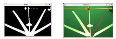
(a) Green binary image (b) Result **Fig 3**. Vision system with shape of ball
