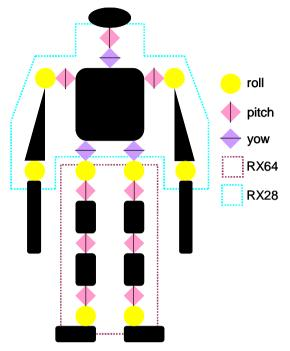
Fig 2. DOF of the robot
