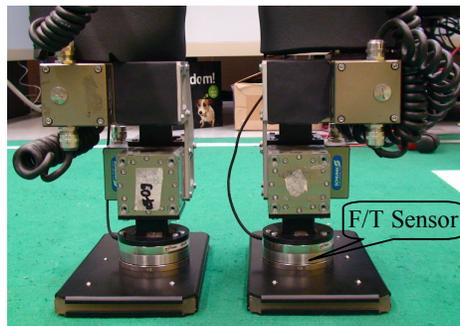
Fig. 6. Force/Torque sensors in the ankles.
