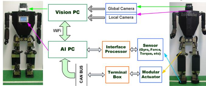
Fig. 1. Block diagram for RESr-III hardware control.
