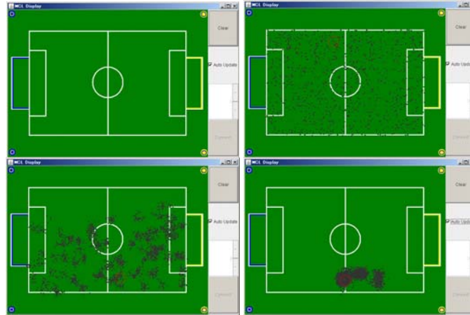
Fig.4 Estimating Process Using Particle Filter
