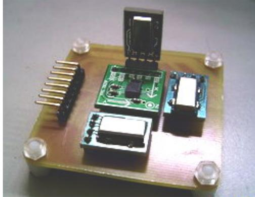
Fig. 6. The photo of accelerometer and gyroscopes.
