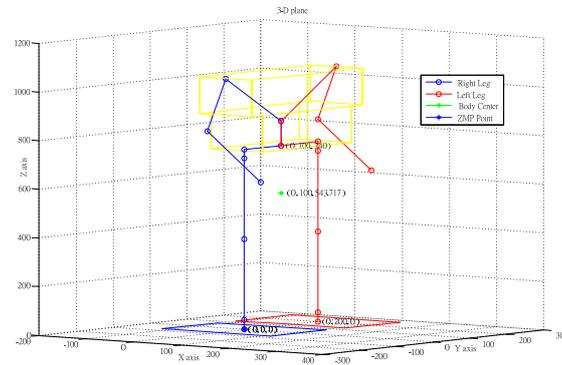
Fig. 1. The kinematic design of a humanoid robot.
