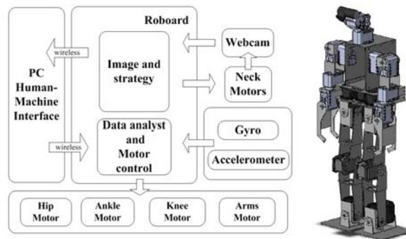
Fig. 3. Block diagram of TWNHR-VI's electrical system
