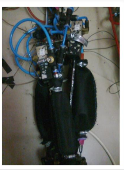
Fig 4: Pneumatic Muscles in Action in the leg area.
