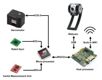
Fig. 2. Robo-Erectus Architecture
