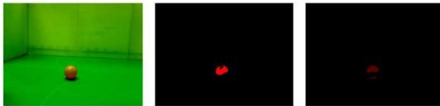
Fig. 6. Evaluated image (left), HSV thresholding (middle), color scoring (right)
