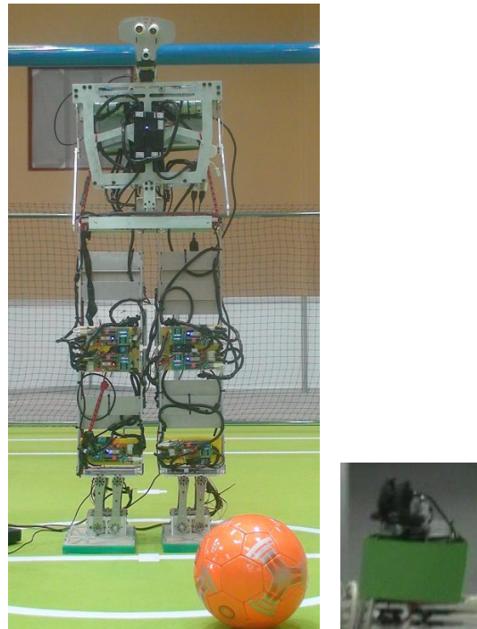
Fig. 4. Photos of assembled HuroEvolution AD (left-hand-side) and the active vision sensor (right-hand-side)
