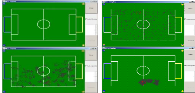
Fig.4 Estimating Process Using Particle Filter
