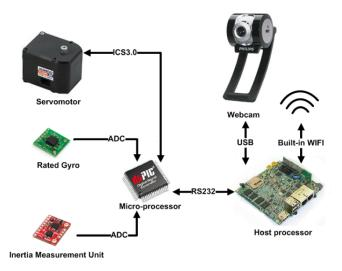
Fig. 2. Robo-Erectus Architecture
