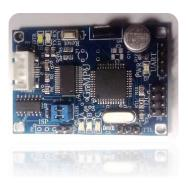
Figure 2. 9DOF IMU
