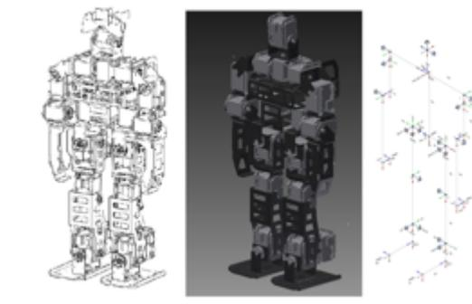
**Figure 3.** Kinematic diagram of the DARwIn-OP based prototype.
