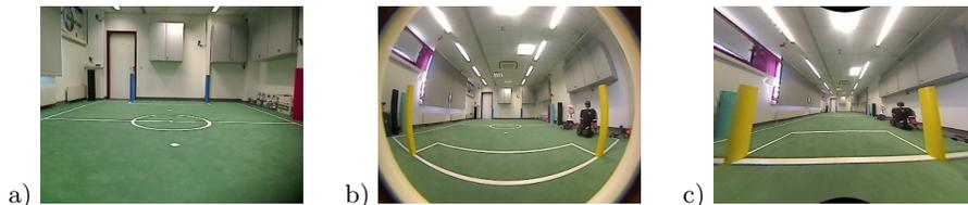
**Fig. 2.** Wide-angle lens: a) A raw camera image of a RoboCup soccer field without the wide-angle lens. b) An image from the same perspective using the wide-angle lens shows the increased field-of-view and the introduced barrel distortion. c) Undistorted camera image.
