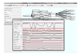
Our custom flow graph visual programming framework is structured by a oriented network of interconnected blocks. From inputs to outputs blocks, signals goes through several filters as gain, PID, signal sum, offset, etc... scheduled at 50Hz.
