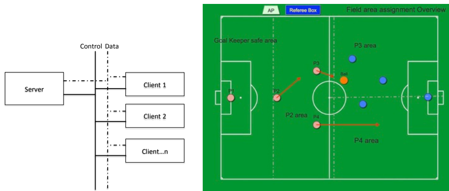
Figure 5. Client-server configuration for inter-robot communication and field area assignment
