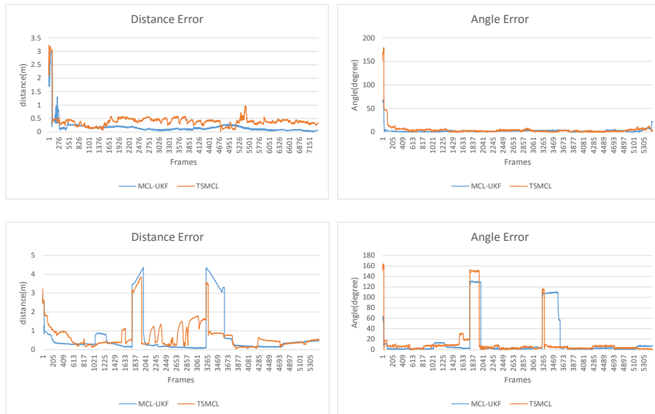
Fig. 2- Results of the accuracy and relocalization experiments. Top row shows the accuracy and bottom row shows the ability to recovering from kidnap.
