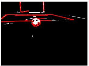
Fig. 2 Binarized image with detected contours
