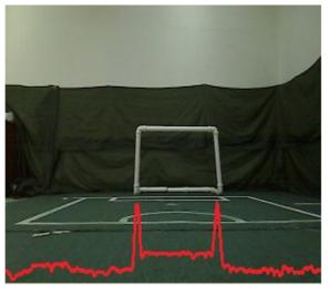
Fig. 7 Histogram of oriented gradients over image
