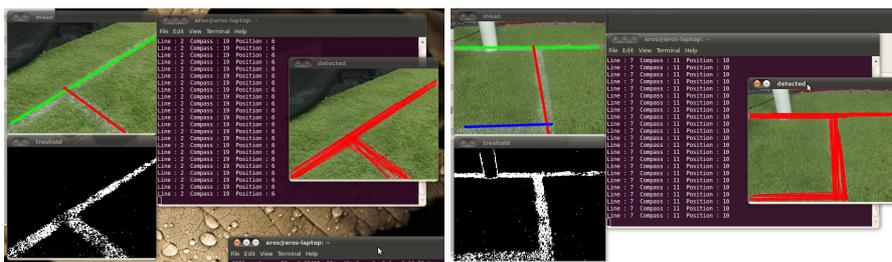
Figure 5. Object segmentation approach by using Hough transform to detect objects on the field line.
