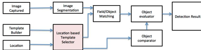
Figure 4. Object detection system using location based template matching approach.
