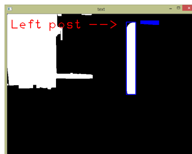
(b) The crossbar is detected (colored in blue), and the algorithm detects that the post in the image is the left post.
