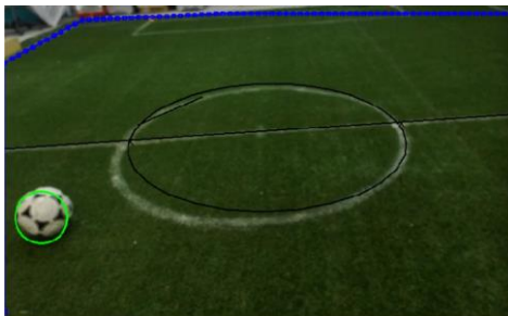
Figure 6. Line and ball detection using edge-based methods
