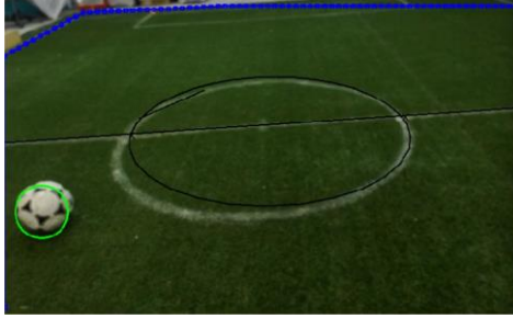
Figure 6. Line and ball detection using edge-based methods
