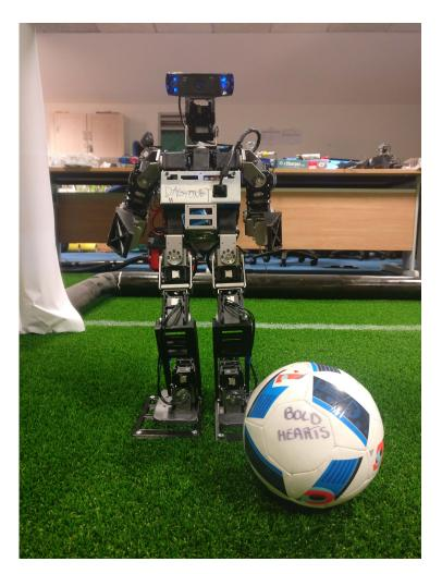
Fig. 2: An example of the new platfrom "Boldheart 2": It has been assembled with a new computational unit (Odroid-XU4), a new camera (Logitech HD Pro Webcam C910) and self-designed torso, feet, arms, legs and a head.
