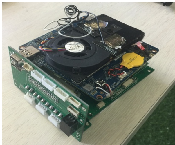
Fig. 3 Electric control system of SYCU-Legendary robot
