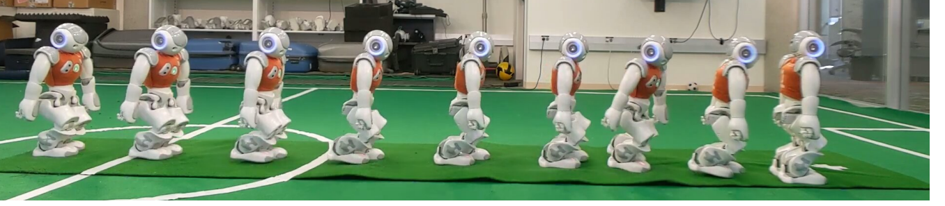
Fig. 1: Experiment setup showing a robot walking on the uneven ground. The NAO begins walking 40 cms behind the center of the circle and walks 300 cms towards the white penalty cross. This image shows a successful walk executed by the robot at 2 sec intervals, learned using the proposed SGAT algorithm.
