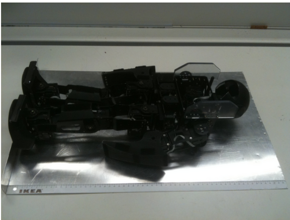
(a) Laying robot upright on measurement device.
