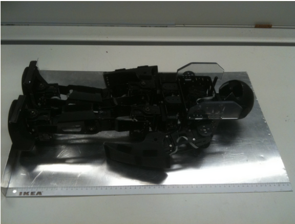
(a) Laying robot upright on measurement device.
