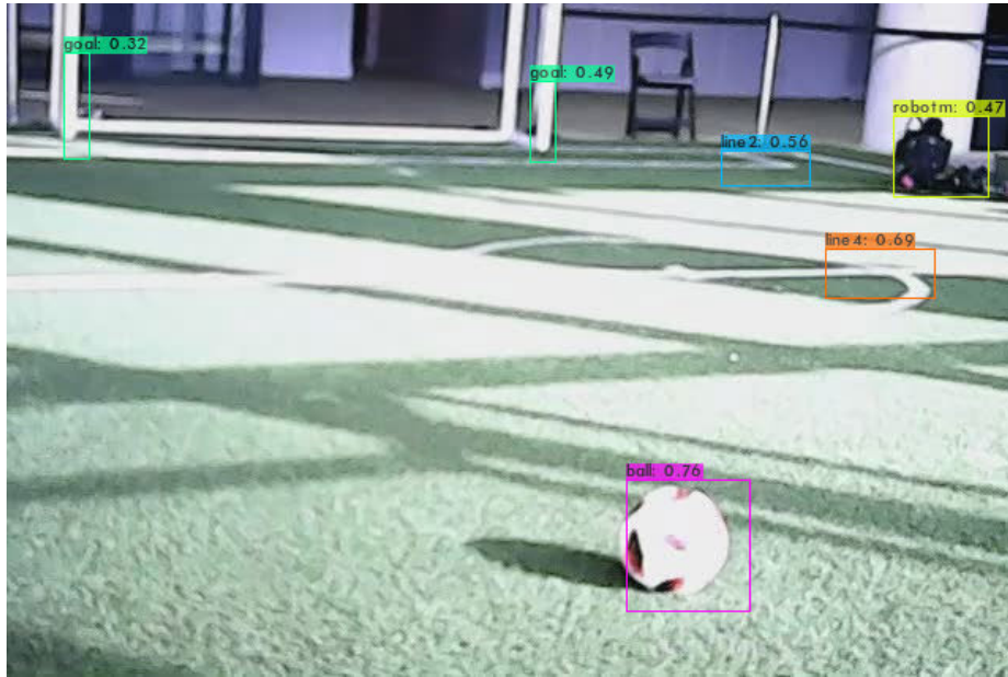
Fig. 3. xYOLO network predictions, showing detections for the ball, goal, line crossings and a robot. Detections in a single frame may be missed or not accurate, but we aim to detections quickly and often.
